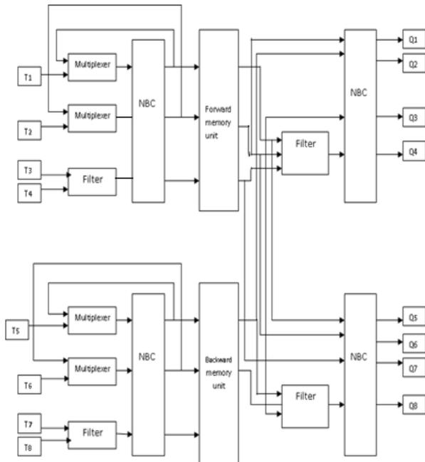
Fig. 8: Trellis check node unit decoding architecture with permutation network
