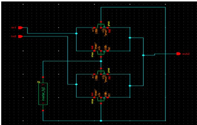
Fig. 6: Multiplexer for the permutation network
