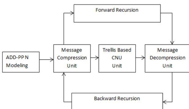
Fig. 1: Block diagram of trellis based decoding architecture
