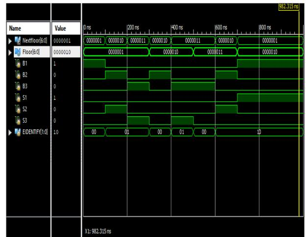
Fig. 8: Elevator Moving from Floor 2 to Floor 1.
