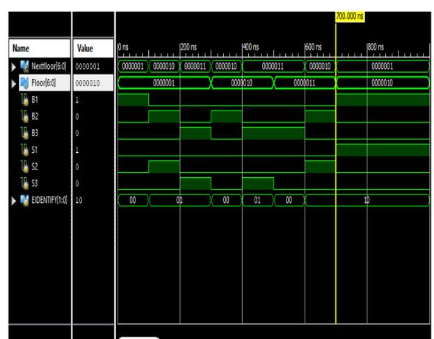
Fig. 10: Elevator Moving from Floor 3 to Floor 2.
