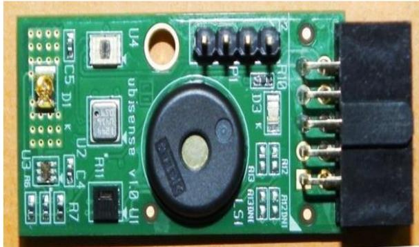
Fig. 3: Ubisense Onboard Sensor Components.
