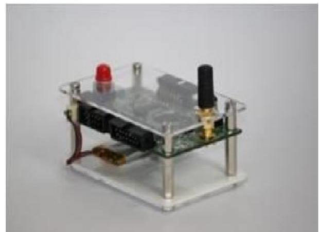
Fig. 2: MSP430 C-Mote Embedded Boards with Sensor Node Arrangement.
