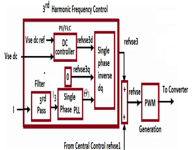
Fig. 5: Control Block Diagram of Series Converter.
