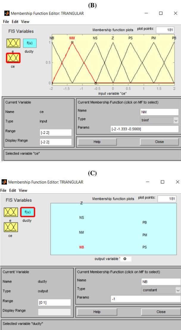
Fig. 6: Membership's Functions of FLC For DC Controller/Current Controller for Series and Shunt Converters of DPFC, (A) Error (E), (B) Change in Error (Ce), Aand (C) Output (O).
