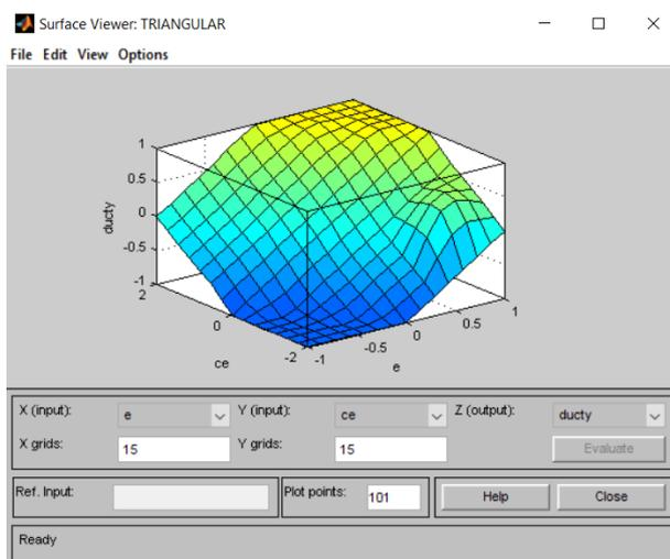
Fig. 7: Graphical Three-Dimensional (E, Ce and O) Surface View of Mmembership's Functions of FLC for DC Controller/Current Controller for Series and Shunt Converters of DPFC.
