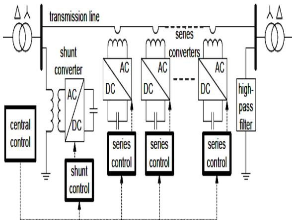
Fig. 4: Control block diagram of DPFC.
