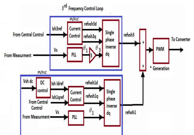
Fig. 8: Control Block Diagram of Shunt Converter.
