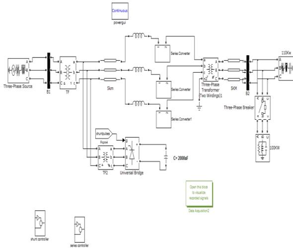
Fig. 11: MATLAB/Simulink Model of Two-Bus System with DPFC.
