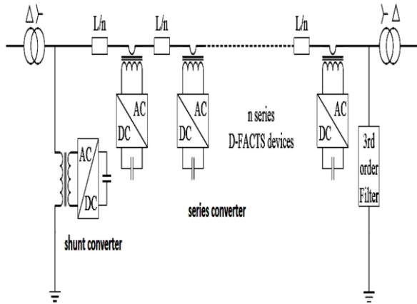
Fig. 1: Distributed Power Flow Controller.
