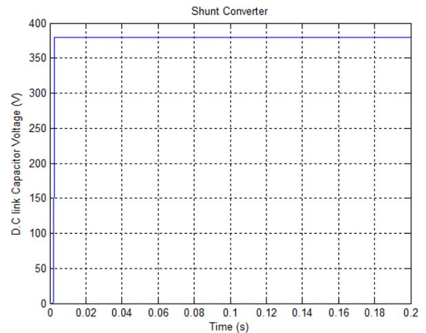
**Fig. 21:** D.C Link Capacitor Voltage of Shunt Converter Using FLC.
