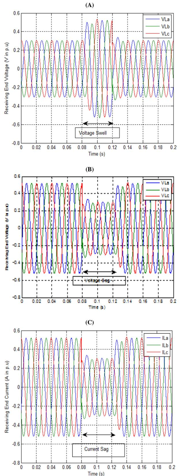
**Fig. 10:** Simulation Results of Two-Bus System without DPFC, (A) Bus-2 Voltage in Swell, (B) Bus-2 Voltage in Sag And (C) Bus-2 Current in Sag.
