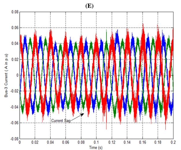
**Fig. 15:** Performance of Three-Bus System with No DPFC, (A) MATLAB/Simulink Model, (B) Bus-2 Voltage, (C) Bus-2 Current, (D) Bus-3 Voltage and (E) Bus-3 Current
