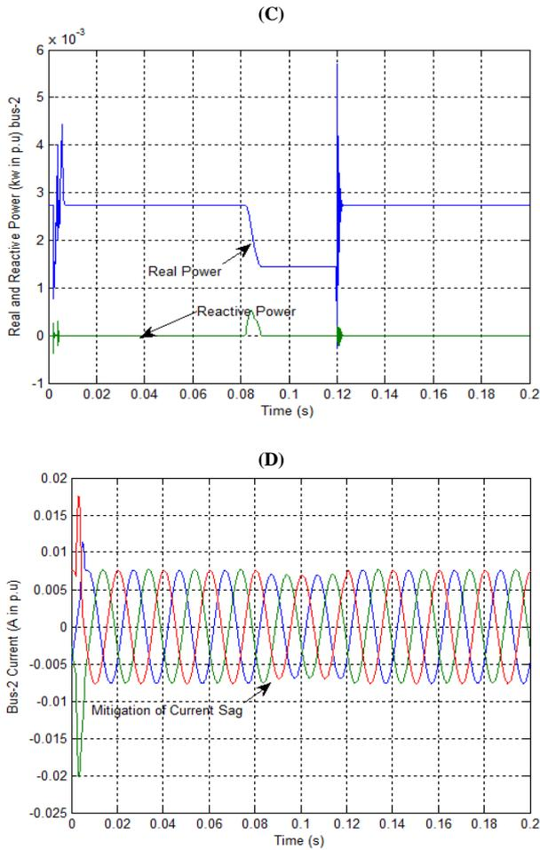
**Fig. 17:** Performance of Three-Bus System with DPFC Using FLC, (A) Bus-2 Voltage, (B) Bus-3 Voltage and (C) Real and Reactive Power at Bus-2 and (D) Bus-2 Current
