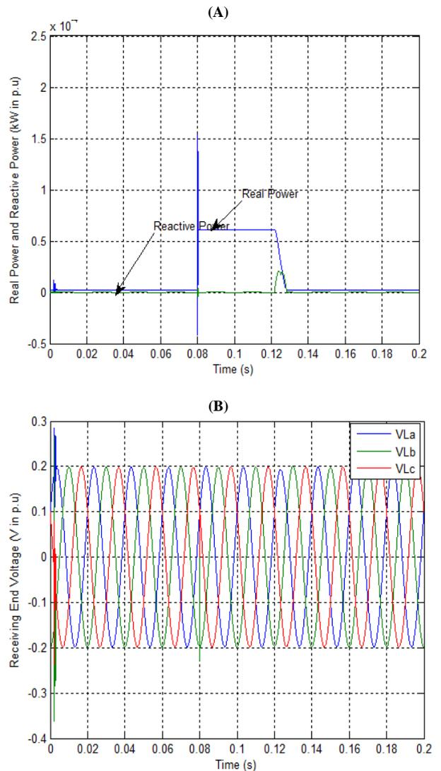
Fig. 14: Simulation Real/Reactive Powers Bus-2 Voltage Results of DPFC with FLC.
