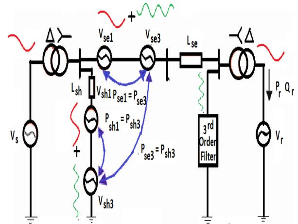
Fig. 2: Simplified Equivalent Circuit of DPFC in Two Bus Power System.
