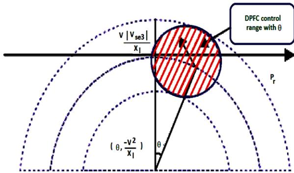
Fig. 3: DPFC Real and Reactive Power Control Range Using Transmission Angel.
