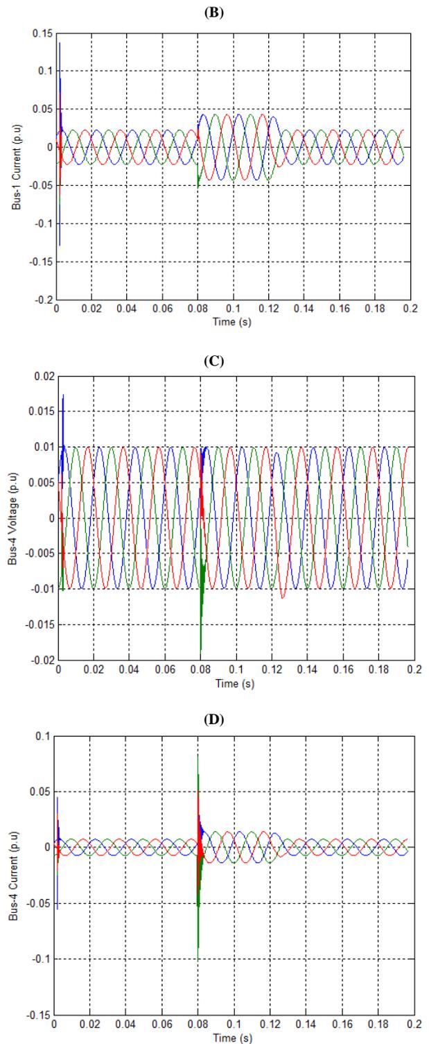
**Fig. 19:** Performance of Five-Bus System with DPFC Using PI Controller, (A) Bus-1 Voltage, (B) Bus-1 Current, (C) Bus-4 Voltage and (D) Bus-4 Current.
