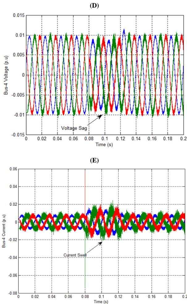
**Fig. 18:** Performance of Five-Bus System with No DPFC, (A) MATLAB/Simulink Model, (B) Bus-1 Voltage, (C) Bus-1 Current, (D) Bus-4 Voltage and (E) Bus-4 Current
