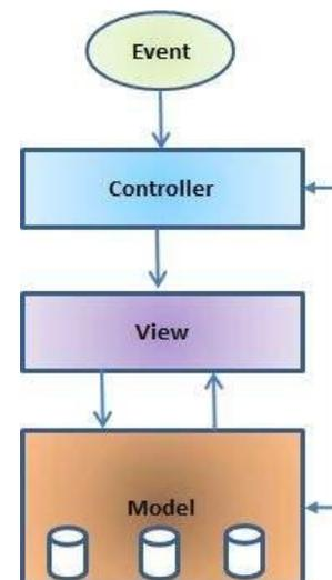
MVC is the interface layer and gives the rising factor to the separation of concerns. the controller will receives all requests for the works and the application and with design to the data needed by the displaying factor. The displaying factor can uses the data prepared by the controlled to evaporate a final presented response.
