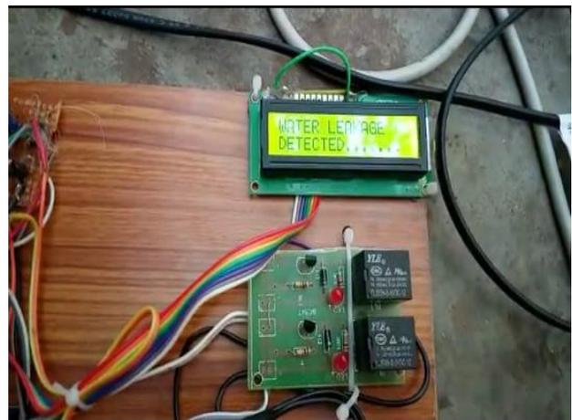
**Fig.6** Water leakage detected show in LCD
