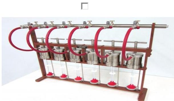
Fig. 4: Low Temperature Low Pressure Filter Press.
