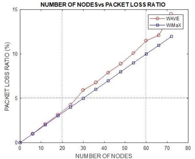
Fig. 6: Graph representing Packet Loss Ratio and number of nodes for WAVE and WiMAX
