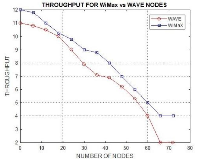
Fig. 5: Graph of Throughput for number of vehicles for WAVE and WiMAX
