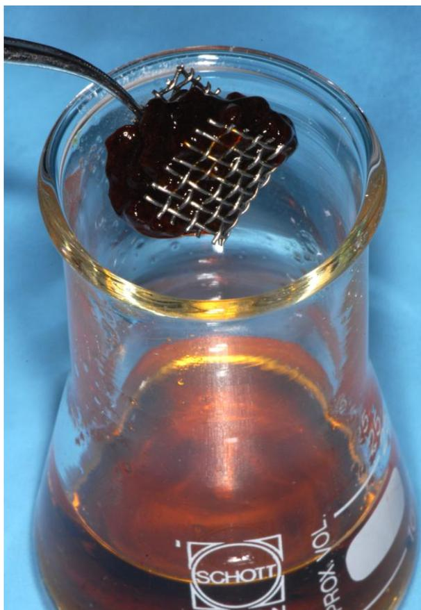
Fig. 1: Illustration of the custom-made mesh made of stainless steel, which served for material transfer and stable immersion.
