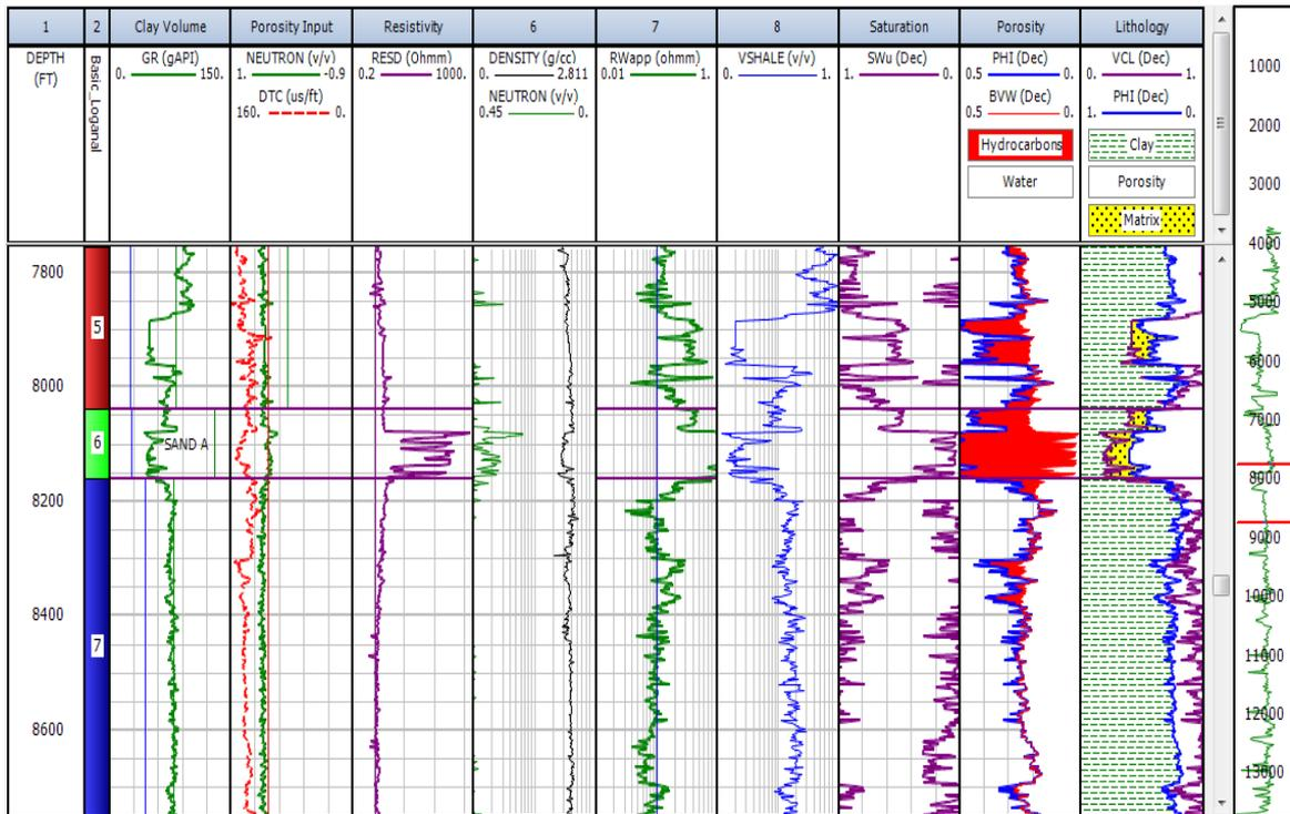
**Fig. 5:** Log Interpretations for Well Bonga 01 Showing Main Hydrocarbon Bearing Interval (Red Color).
