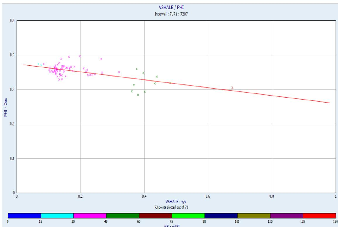
Fig. 14: Cross plot of Porosity and Shale Volume within the Reservoir Unit Showing High Porosity for the Clean Sand Unit.
