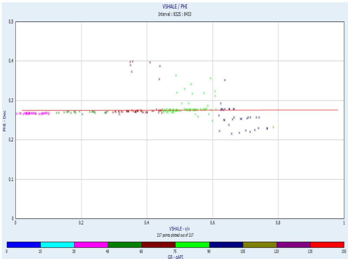
Fig. 10: Cross plot of Porosity with Vshale Showing High Correlation for Clean Sands Up to 58 API Reading.
