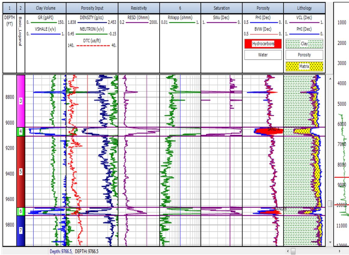
**Fig. 11:** Log Interpretations for Well Bonga 08 Showing Main Hydrocarbon Bearing Interval (Red Color). This Log Interpretation Shows Evidence of Stacked Reservoir in the Well Location. Sand B Has the Highest Porosity Value for the Five Wells, 2634 Md.
