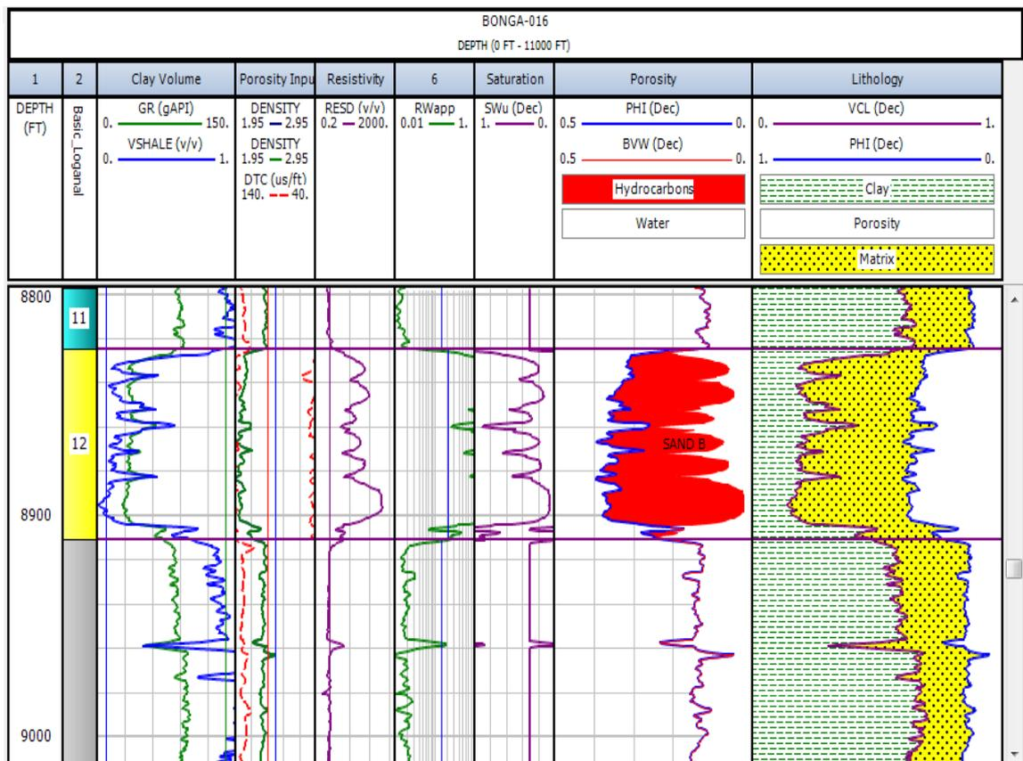
**Fig. 13:** Log Interpretations for Well Bonga 16 (Sand A) Showing Main Hydrocarbon Bearing Interval (Red Color). This Log Interpretation Shows Evidence of Stacked Reservoir in the Well Location.
