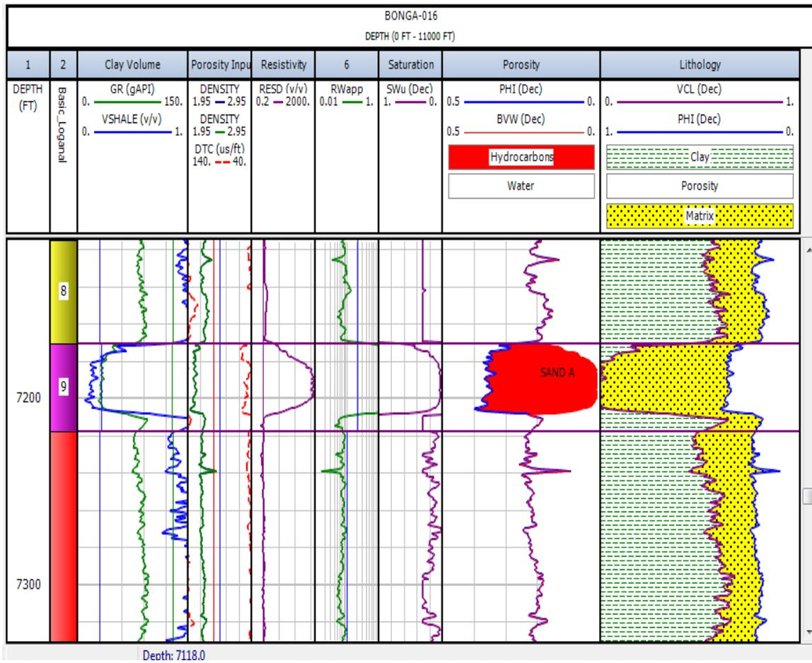
**Fig. 13:** Log Interpretations for Well Bonga 16 (Sand A) Showing Main Hydrocarbon Bearing Interval (Red Color). This Log Interpretation Shows Evidence of Stacked Reservoir in the Well Location.
