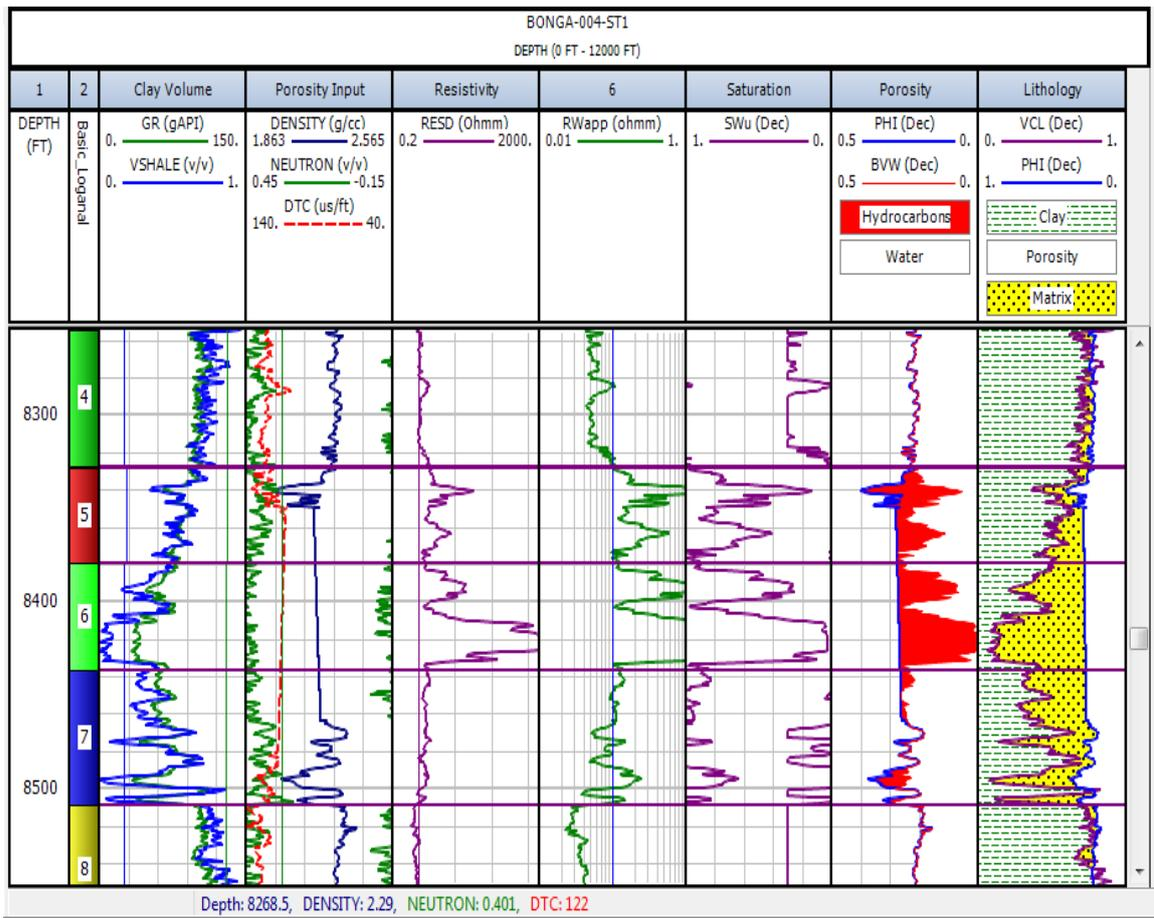
Fig. 9: Log Interpretations for Well Bonga 04 Showing Main Hydrocarbon Bearing Interval (Red Color). Density Data Quality at Reservoir Unit was Unreliable.
