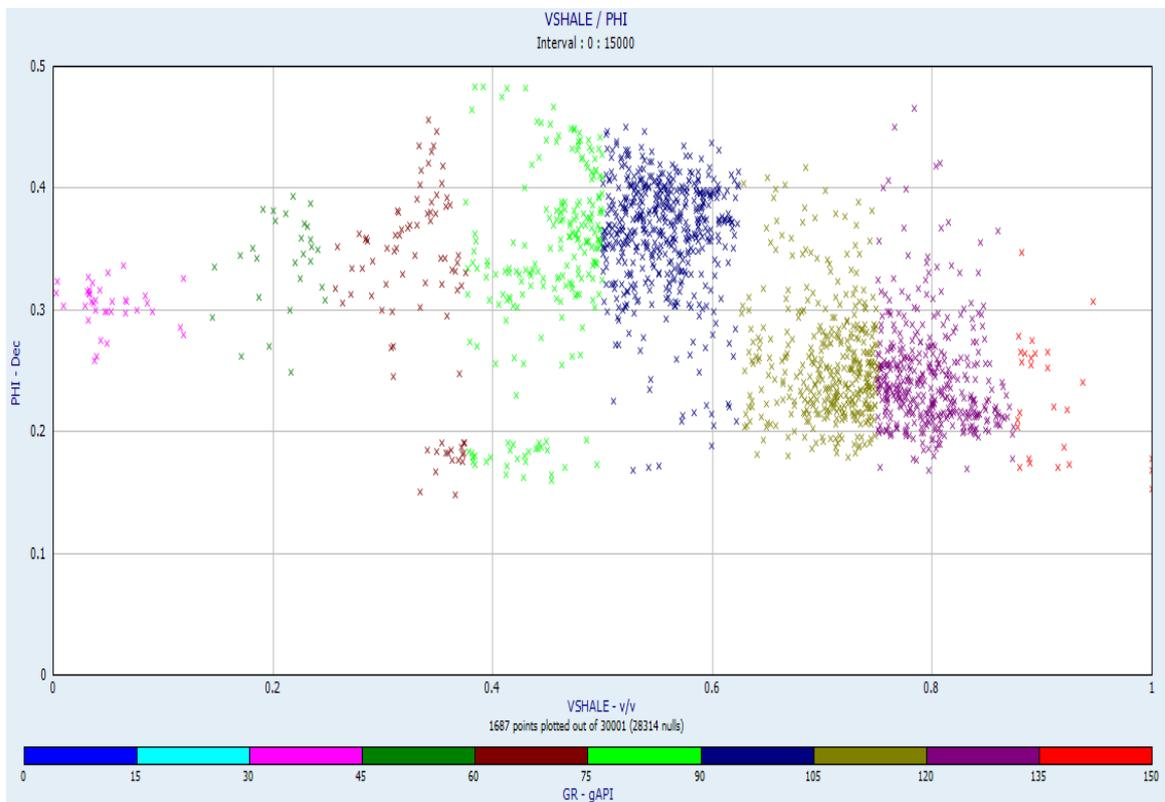
Fig. 8: Cross plot of Porosity with Volume of Shale for the Whole Well Bonga 02 Showing Range of Porosity Values with Highest Porosity at 0.40 to 0.45. Permeability Value at Reservoir Unit Is 770 Md.
