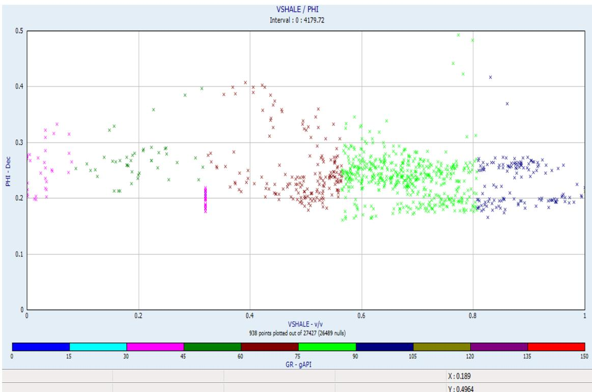
**Fig. 6:** Cross plot of Porosity and Volume of Shale for Bonga 1 Showing the Range of Porosity Values with  $V_{shale}$  for the Entire Well.
