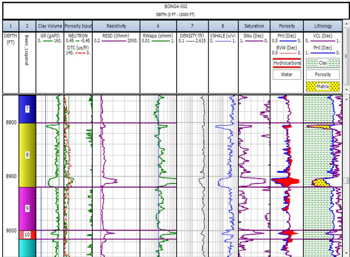
Fig. 7: Log Interpretations for Well Bonga 02 Showing Main Hydrocarbon Bearing Interval (Red Color). Thin Sand with High Permeability Value Is Indicated in Red.
