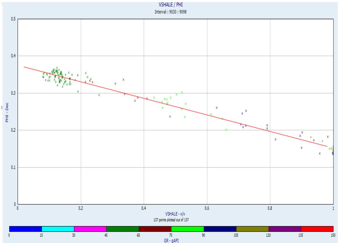
**Fig. 12:** Cross plot of Porosity with Vshale Showing High Correlation for Sands within the Reservoir Unit. This Reservoir Demonstrates Effect of Shale Content on Porosity and Permeability.
