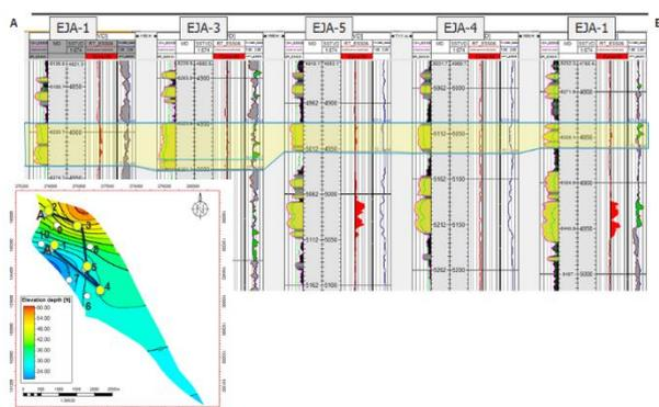
Fig. 20: E-15 Reservoir Stratigraphic Cross Section.
