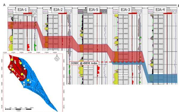
Fig. 18: E-15 Reservoir Original Structural Cross Section.
