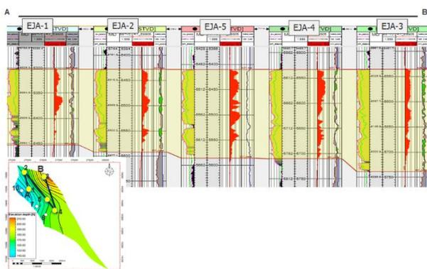
Fig. 19: E-21 Reservoir Stratigraphic Cross Section.
