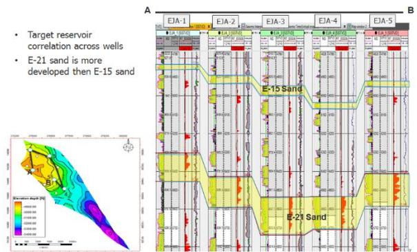
**Fig. 8:** Structural Cross Section through Target Sands.
