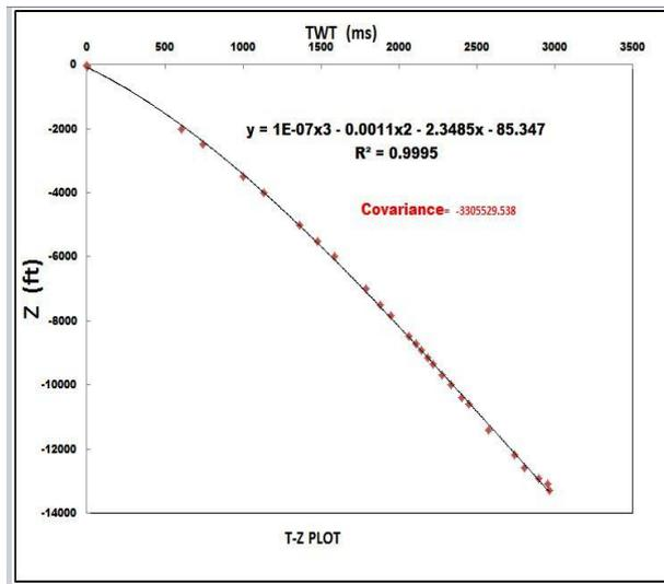
Fig. 12: Time-Depth Plot Used in the Time-Depth Conversion.
