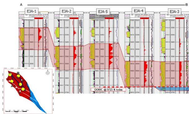
Fig. 16: E-21 Reservoir Original Structural Cross Section.
