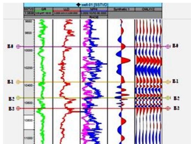
**Fig. 9:** Seismic to Well Tie Showing A Relatively Good Well to Seismic Tie.
